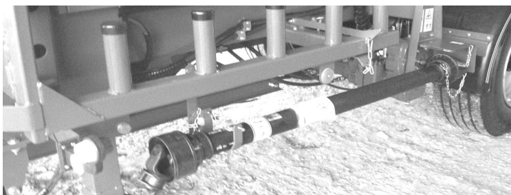
PTO - axle in transport mode
